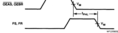
Waveform 2. Propagation Delay, Output Enable to Flag Output
